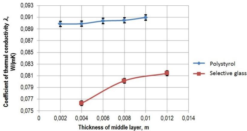
Fig. 8. Thermal conductivity coefficient  $\lambda$  ( $W \cdot m^{-1} \cdot K^{-1}$ ) values for the samples with organic glass (polystyrol) and inorganic glass with selective coating in the middle layer
