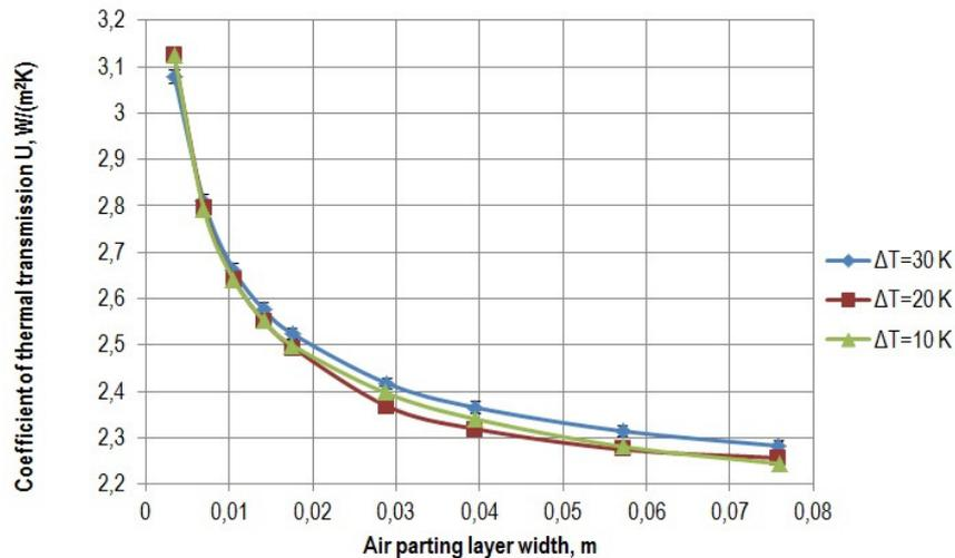
Fig. 5. Dependence of the thermal transmission coefficient on the width of the air separation layer, the values of the coefficients of thermal transmission are calculated
