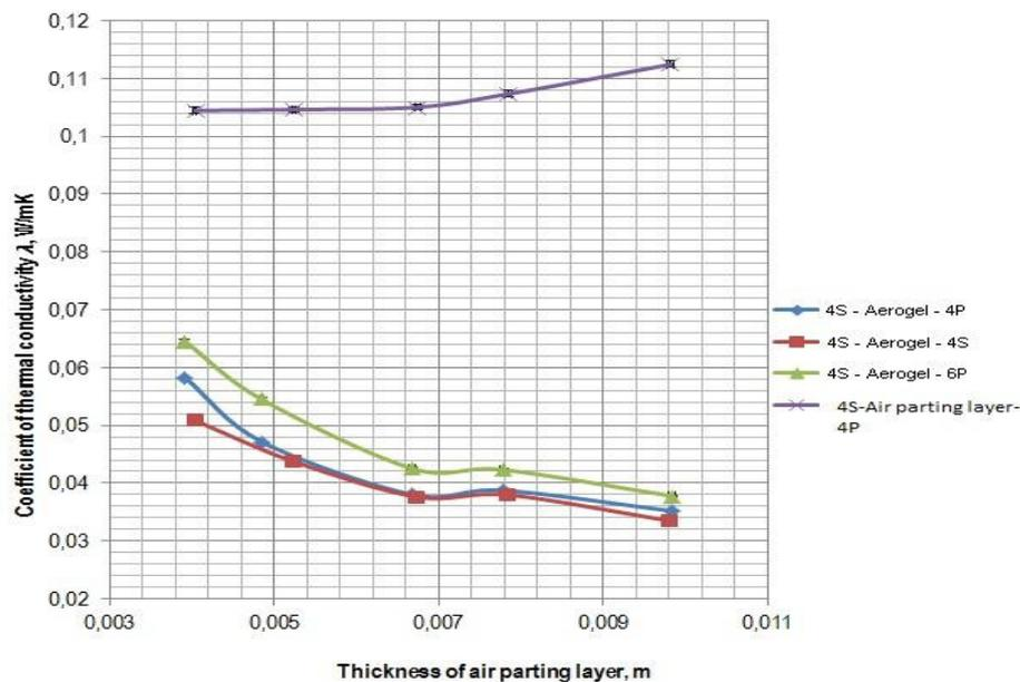
Fig. 6. Thermal conductivity coefficient  $\lambda$  ( $\text{W}\cdot\text{m}^{-1}\cdot\text{K}^{-1}$ ) values of the samples with aerogel filling and air parting layer
