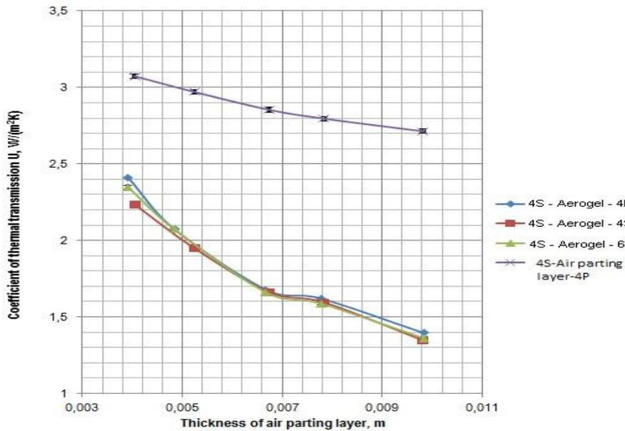
Fig. 7. Thermal transmission coefficient  $U$  ( $W \cdot m^{-2} \cdot K^{-1}$ ) values of the samples with aerogel filling and air gap (calculated)
