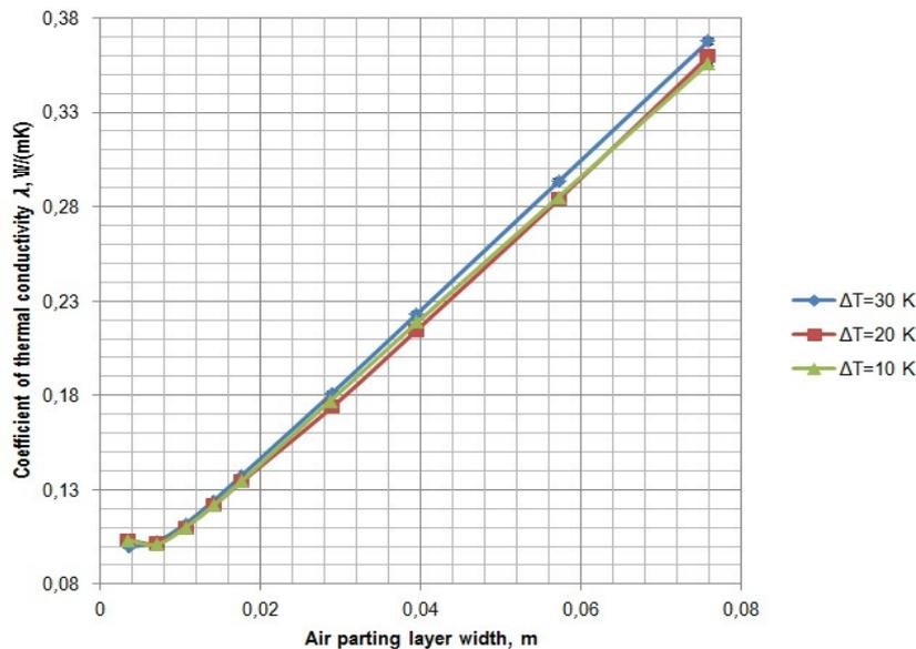
Fig. 4. Dependence of the coefficient of thermal conductivity on the air parting layer width for a horizontally positioned sample
