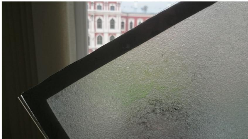
Fig. 1. Sample with aerogel – 4S-4A-4P (the authors’ photograph)
